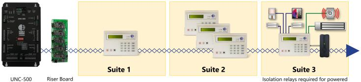
olation relays required for powered outputs. Ordered separately.
