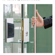
Operating Modes The KP-6840 can be used for Card + PIN, PIN + Card, Card Only, or PIN Only. Mode selection is made by programming the host system, not by selection in the KP-6840.
