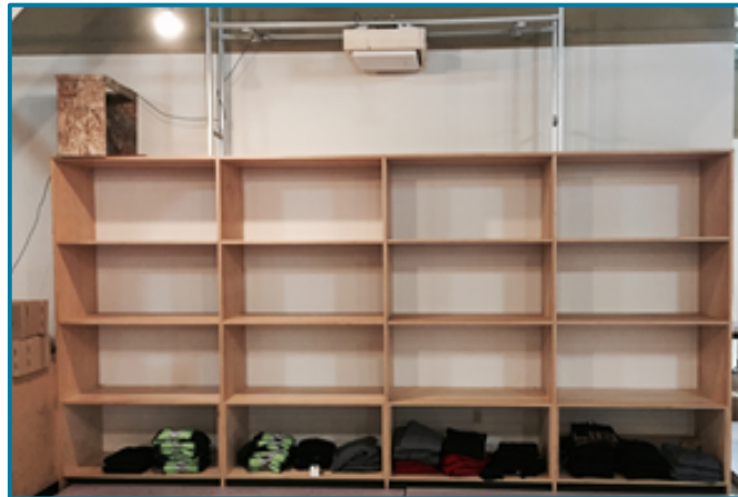
Placement next to wall and directly above shelving makes the bottom shelf items difficult to read for the xArray.
